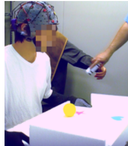
Fig. 1 Appearance of experiment by ATR [1]: The participant grabs the tray with both hands and the experimenter passes the object from the right side to the third hand in the center.
